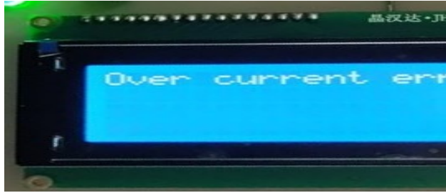
Figure 2.2 Over Current Fault
